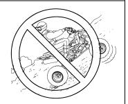
If the ATV begins rolling backwards: Keep weight uphill. Never apply engine power. Never apply the rear brake while rolling backwards. Apply the front brake slowly. When fully stopped, apply rear brake as well, and then lock the parking brake. Dismount on uphill side, or to either side if pointed straight uphill. Use the K-Turn to turn the ATV around and remount. See page 86.
